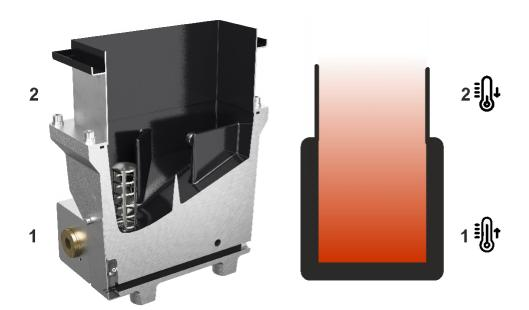
Baumer hhs has used a different approach by introducing a two-zone tank. This innovative design divides the tank into two zones: a heated lower zone where the adhesive reaches its processing temperature and an unheated upper zone where the hot melt slowly softens at a lower temperature. This unique setup creates a temperature gradient during operation, providing a cooler protective cover to prevent the adhesive from burning.
