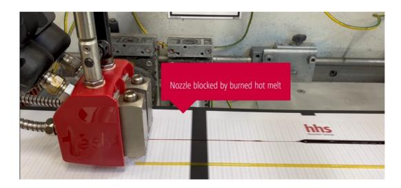
A comparison was conducted between a newly developed hot melt hose featuring a metal core and three different hot melt hoses with a plastic core. Following an equal heating period, noticeable alterations in both the color and viscosity of the hot melt were observed in the plastic core hoses, while the hot melt in the metal core hose remained unchanged, retaining its initial clarity. These findings are quite straightforward and do not necessitate an intricate scientific explanation.
