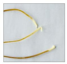
The mystery of the remaining burns was swiftly unraveled. Engineers from Baumer hhs conducted tests on various hot melt hoses to simulate burns. Upon examination, it was revealed that the adhesive around the metal connections showed no signs of burning, while the area around the flexible hose displayed
