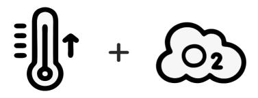
Charring in hot melt systems is a result of the combined presence of heat and oxygen . As heat and oxygen work hand in hand, higher temperatures and increased exposure to oxygen accelerate the charring process. To prevent charring, it is crucial to either reduce the temperature or minimize oxygen contact. These strategies are essential for maintaining the integrity of hot melt systems.
