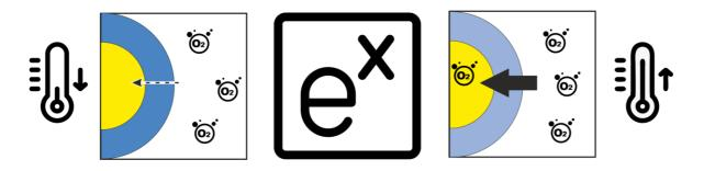
Literature research has demonstrated that oxygen diffusion through thermoplastic tubing undergoes an exponential increase as temperature rises. At room temperature, silicone or PTFE tubing is relatively impermeable, but at higher temperatures, it exhibits significant permeability. This poses a critical concern as a small amount of hot melt comes into contact with a large internal surface area of the tubing.
